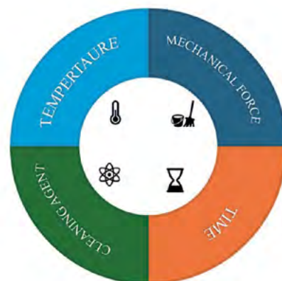
Figure 2 Sinner's circle, or the balance of four factors essential for cleaning, namely cleaning agent, time, temperature and mechanical force (Sinner, 1960)
