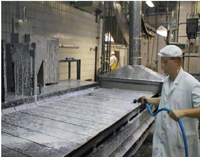
Figure 3 Use of foaming agent in a slaughterhouse (Source: Dulikravić, 2019)
