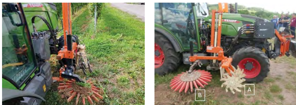
Figure 2. Mechanical weed control with a rotary star tiller (A) and finger weeder (B)
