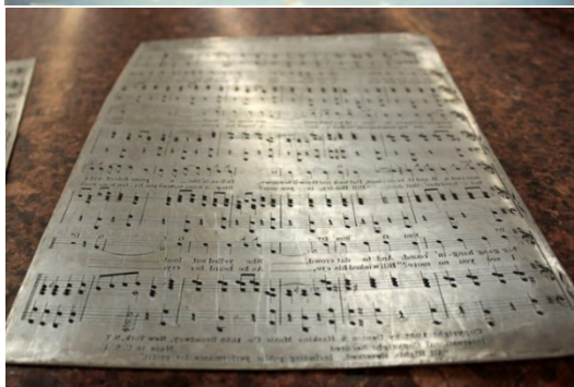
Figure 9 Monolithic printing form made of: a) wood [56], b) metal [57]
