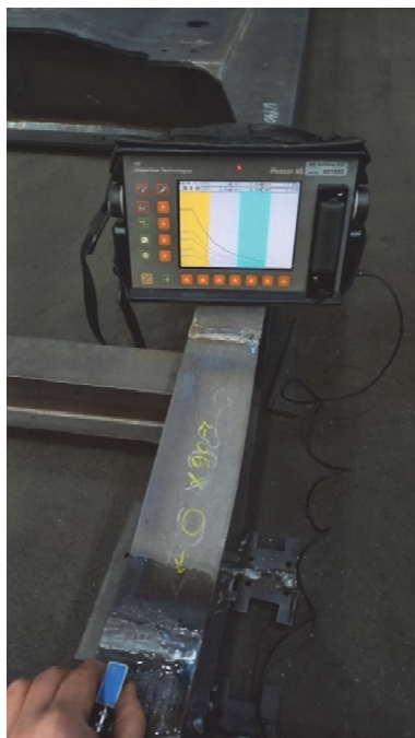
Figure 18 A scan of the defect located in the root of the weld no. 11
