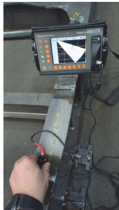
Figure 20 S scan of the defect located in the root of the weld no. 10
