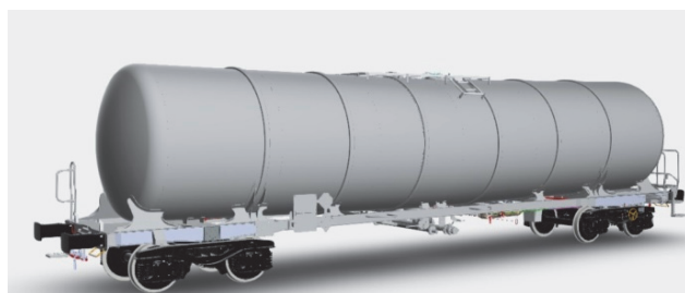
Figure 1 3D model of Zacns 98 m 3 wagon
