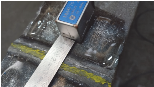
Figure 16 Marking the defect in the filled area of weld no. 1
