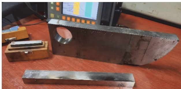
Figure 9 UT device GE Phasor HS and accompanying calibration samples
