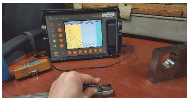
Figure 10 Calibration sample used for sensitivity configuration
