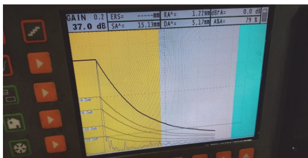
Figure 11 Final form of DAC curve
