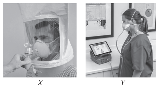
Figure 2. Illustration of a qualitative test injecting an aerosol into the hood while the wearer performs some speaking exercises (X), and a PortaCount test which is a quantitative mask leakage test comparing particle counts between the inside and outside of the face mask (Y)
