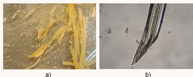
Figure 5. Samples exposed to citric acid in period of 7 days: a) destruction of biocomposite and b) destruction of fibre
