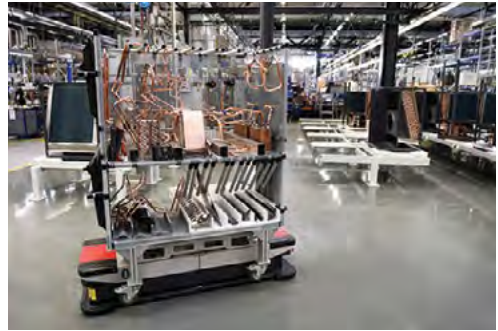
Slika 2. AGV u proizvodnji (Izvor: https://www.igz.com/en/blog/agvs-in-production-supply/ ) / Figure 2. AGV in production supply (Source: https://www.igz.com/en/blog/agvs-in-production-supply/ )
