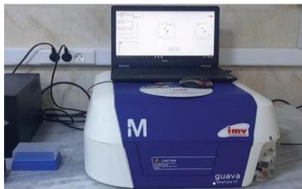
Fig. 4. Guava EasyCyte HT Plus Cytometer (Millipore, USA)
