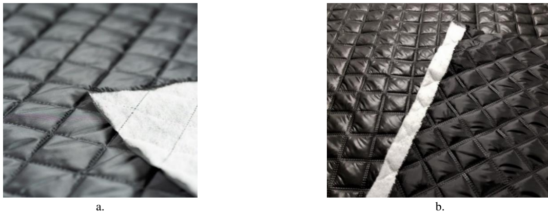
Fig.1 Diamond-shaped quilted lining with a. sewing machine and b. ultrasonic welding technique [3, 4]
