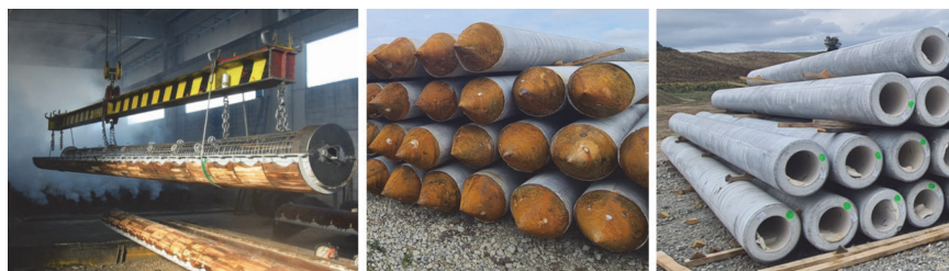
Figure 2. Precast RC piles (design, pile top – steel spike, pile head)
