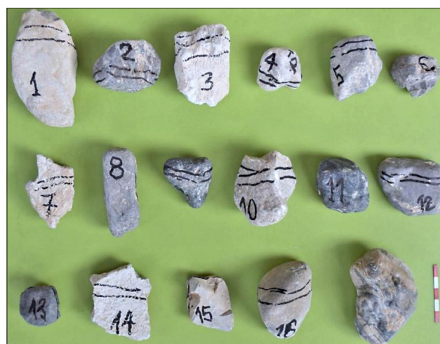
Figure 6. Natural clasts from the Papuča gravel pit prepared for cutting and making thin sections, bottom right scale in centimeters
