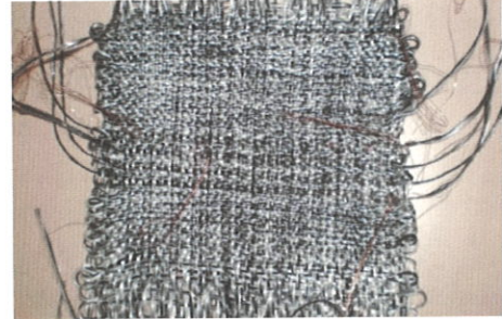
Figure 3. 2D structure with integrated sensors in weft direction [9]
