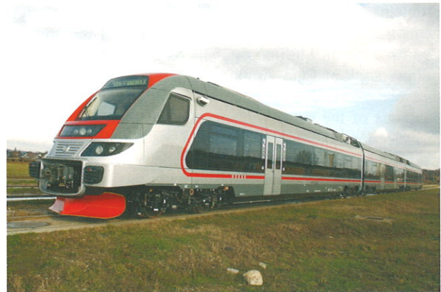
Figure 4. Diesel-electric motor train of TZV Gredelj, Zagreb
