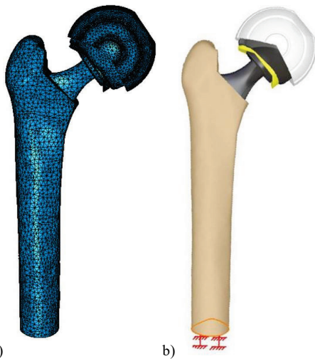
Figure 2 a) Finite element mesh and b) clamp constraint (Endoprosthesis 2)
