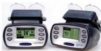
Figure 4 DriftBox GPS measurement device [17]
