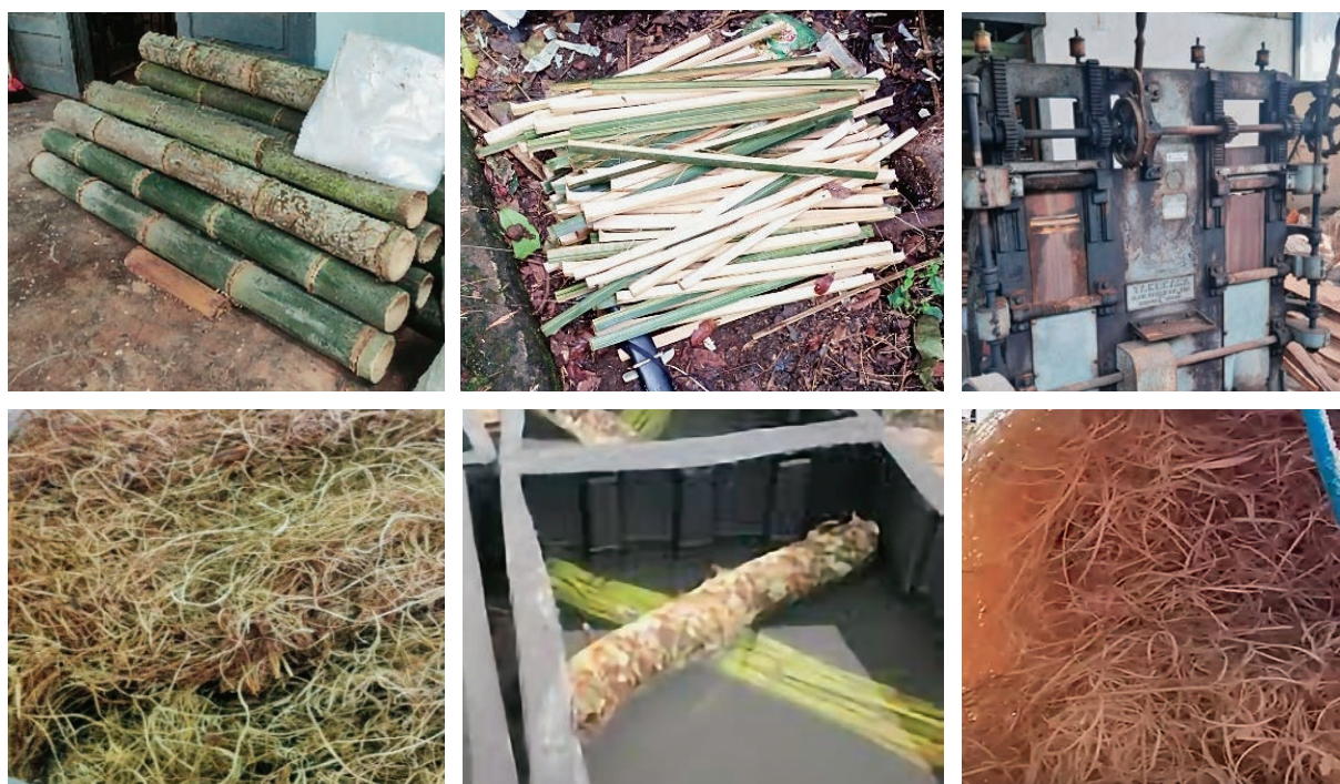
Figure 1 Manufacturing process of bamboo wool: a) bamboo stalks, b) bamboo strips, c) wool-making machine Takekawa Iron Work, d) bamboo wool, e) bamboo wool soaked in cold water, f) bamboo wool after being soaked
