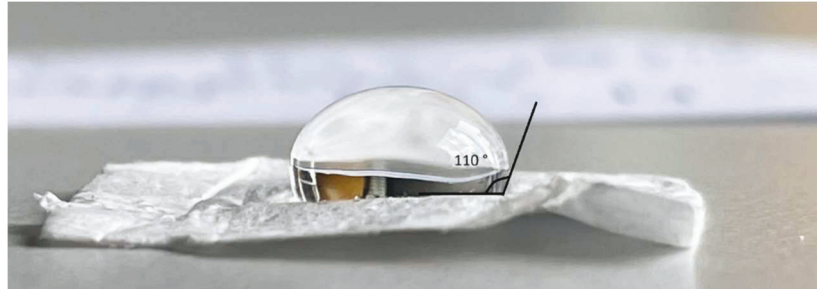
Fig 6 Contact angle of PCL/collagen sample
