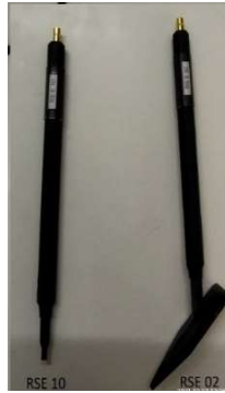
Figure 6. Probes of type ROHDE SHWARZ, probe (1) RSE 02, and probe (2) RSE-10.
