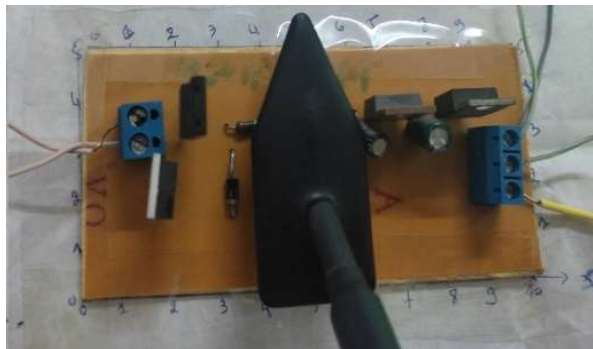
Figure 13. Nearby electric field measurement on the IR2110 driver surface.
