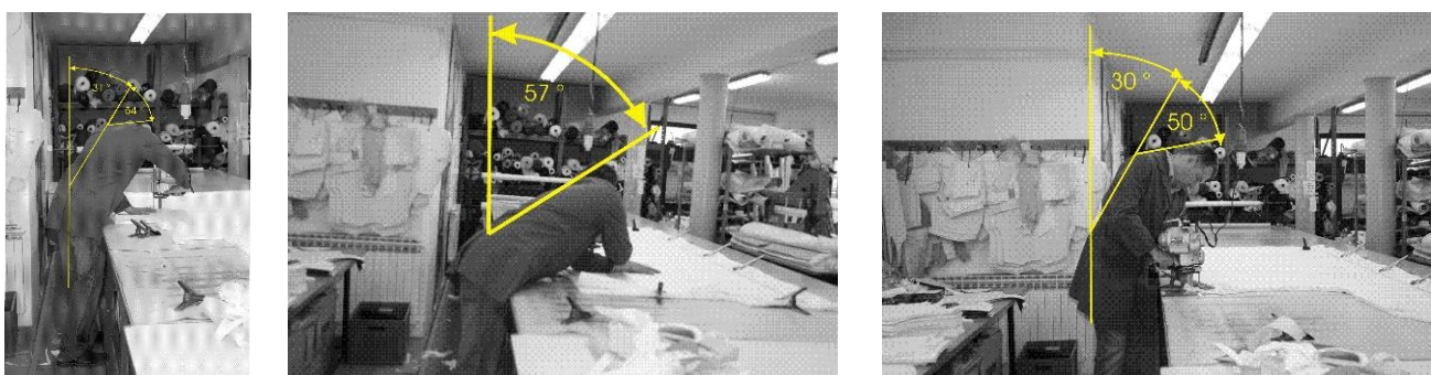
Fig.3 The characteristic working postures when cutting with a straight knife (RM1)
