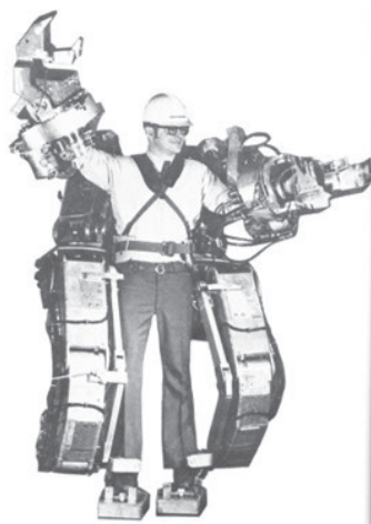
Slika 1. Egzoskelet GE Hardiman I Figure 1. GE Hardiman I exoskeleton
