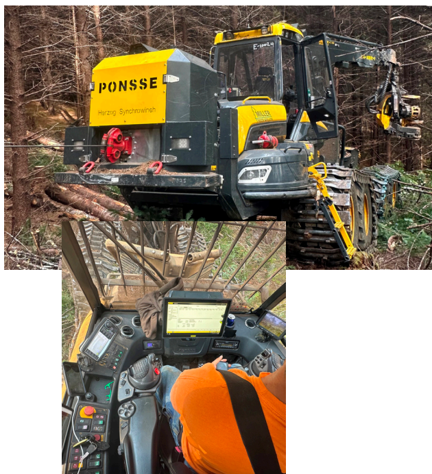
Figure 2 Tethered harvester (up), observation from inside the operator cabin (down).
