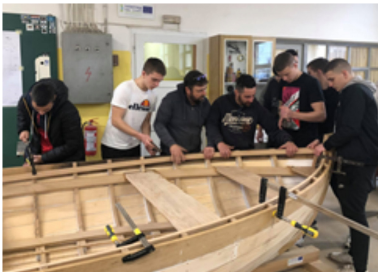
Figure 7. Making a replica of a traditional pasara at the Rijeka Technical School
