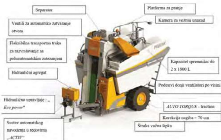
Slika 7. Pregled vučenog kombajna Pellenc 60 (Izvor: https://pellencus.com/wp-content/uploads/2019/08/Pellenc-3d-grapesline )
