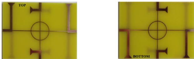
Fig. 7. Fabricated four element MIMO antenna in [40].
