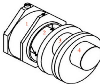
Figure 1. Quality control phantom for CT device Source: Radiology department user manual of the CT device
