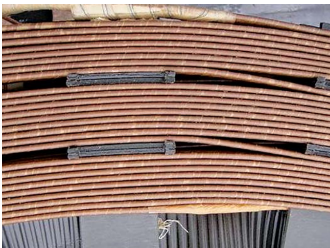
Figure 1. Failure point: wrapped discs (at left), no overwrapping (at right)
