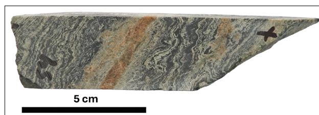
Figure 9. Wiggly textures with black and white bands cut by veins in the shallower part of the deposit. SEM-EDX and petrographic analysis show that the black bands are magnetite with small amounts of cassiterite and wolfram-bearing minerals, while the white bands are fluorite.
