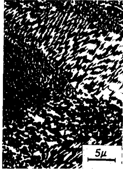
FIG.4: Metastable eutectic \gamma_2 -Al. Deeply etched in KOH. \gamma_2 - white
