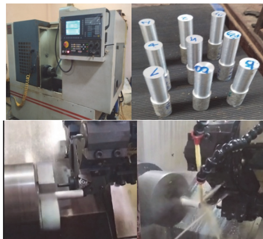
Figure 3 Experimental setup of CNC turning machine (Batliboi Smartturn CNC lathe) and the machined specimens
