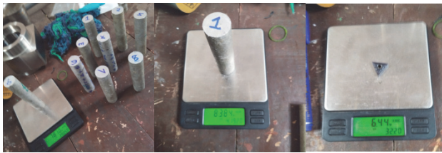
Figure 4 Evaluation of removal rates of tool and workpiece of CNC turned specimen
