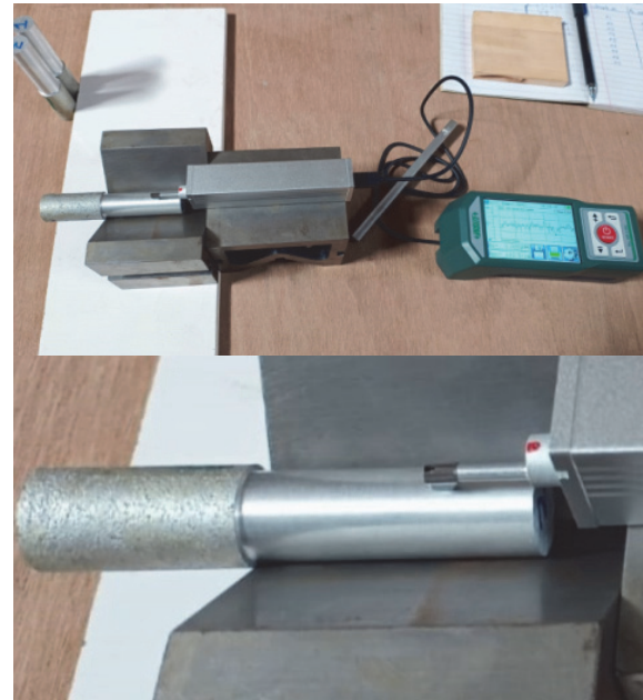
Figure 5 Measurement of stylus probe used for surface roughness testing
