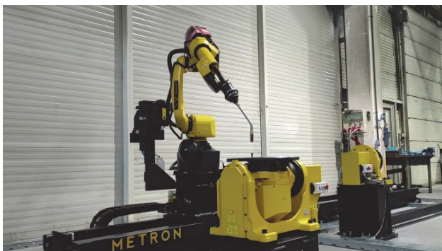
Figure 1 Robotic welding system developed by Metron
