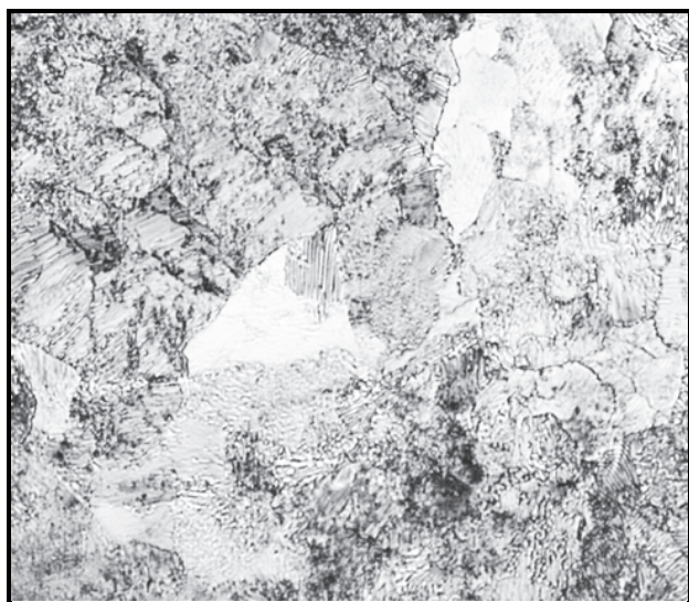
Figure 7 Pearlite microstructure of the base metal of steel rail R260-60E1. Magnification 100x
