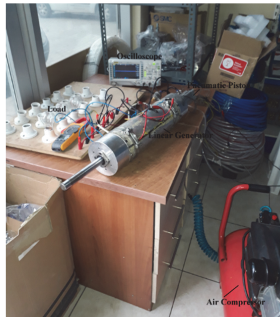
Figure 10 Experimental module of the prototype 9/10 polygonal linear generator with pneumatic system
