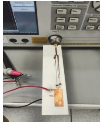
Figure 11 Photograph of the rectifier board under measurement
