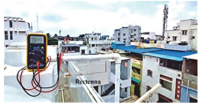
Figure 16 Photograph of rectenna measurement in an outdoor environment on a roof
