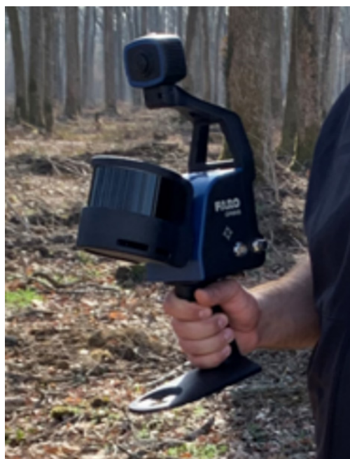
Slika 2. Laserski skeneri korišteni u istraživanju: TLS instrument FARO Focus Premium 150 (lijevo) i PLS instrument FARO Orbis (desno). Figure 2 Laser scanners used in the research: FARO Focus Premium 150 TLS instrument (left) and FARO Orbis PLS instrument (right).
