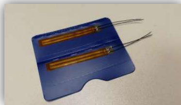
Figure 6. - Strain gauges for concrete
