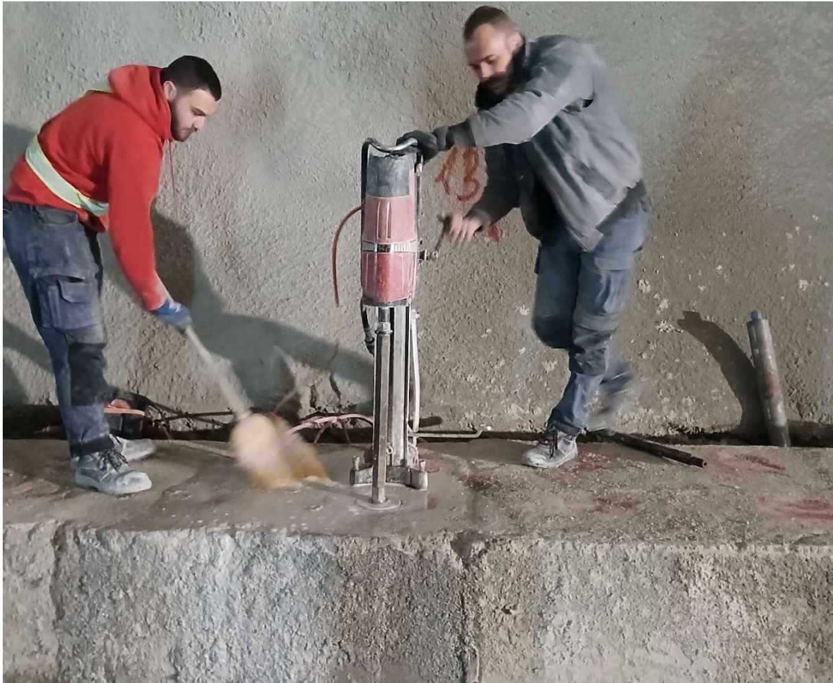
Figure 3. Collection of core samples from locations 1 and 21 and preparation for laboratory tests [photo by authors].
