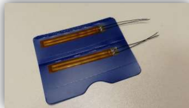
Figure 10. - Strain gauges for concrete
