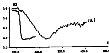
Fig.2. Reflectivity of \text{Pb}_{0.97}\text{Hg}_{0.03}\text{Te} as a function of wavenumber for the samples produced using both Bridgeman (a) and Czochralsky methods.
