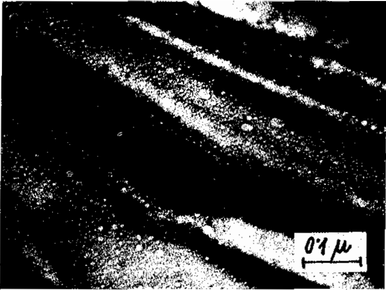
Fig. 3 Coalescence of small argon bubbles in \text{UO}_2 after heating with an intense electron beam in electron microscope ( \text{UO}_2 bombarded with 4 keV \text{A}^+ ions; ion dose 7.5 \times 10^{16} ).
