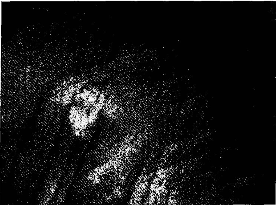
Fig. 9. Cu thin foil bombarded with 5 keV A^+ ions at a dose of 10^{16} ions/cm 2 . Apart of the dislocation segments due to the opening of the loops, another network of dislocation lines is visible, not showing the black and white contrast. These lie thus deeper under the surface and belong to a system of misfit dislocations.
