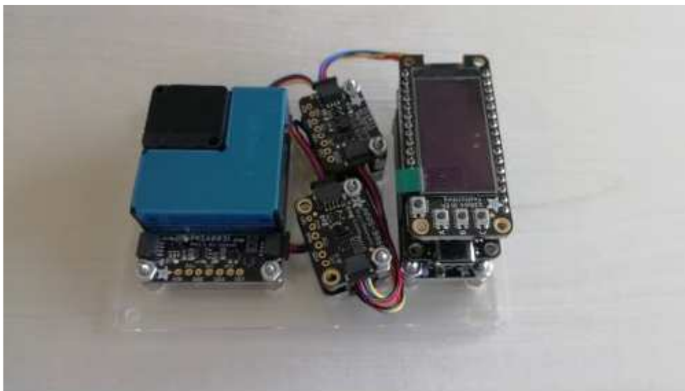
Figure 1. Arduino-based sensor system for air quality monitoring used in the research
