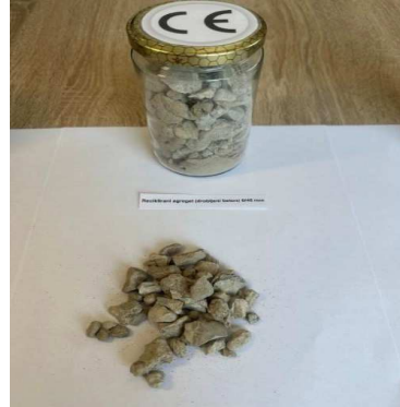
Figure 4. Recycled Aggregate (crushed concrete) 0/45 mm
