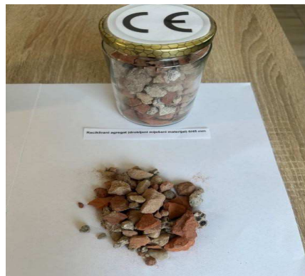
Figure 5. Recycled Aggregate (crushed mixed) 0/45
