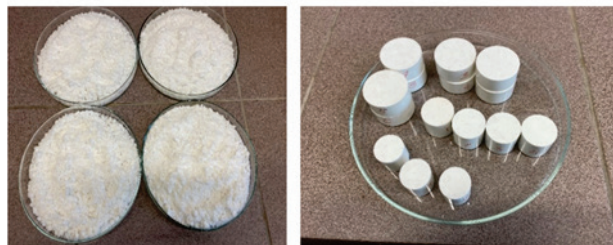
Fig. 12. Samples of TKX-50/Paraffin 97/3 granules before drying (left) and a set of pressed pellets of the same formulation (right) [45].
