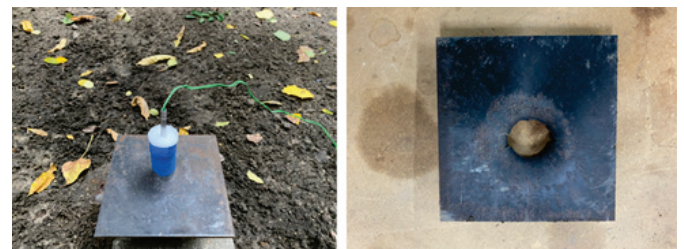
Fig. 9. TKX-50 charge metallized with Al (left) and witness plate after detonation of the TKX-50/Al charge (right) (Klapötke, 2023).
