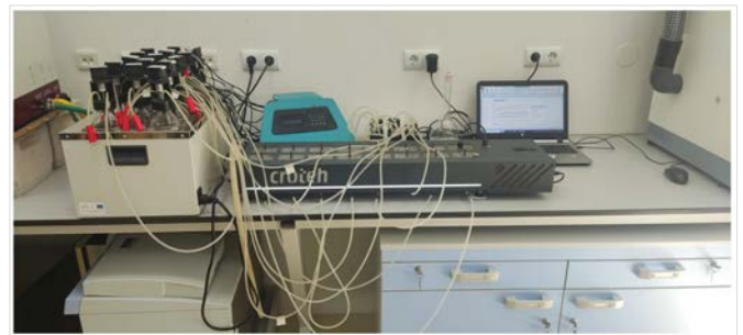
Figure 1. Anaerobic digestion setup for batch biogas production
