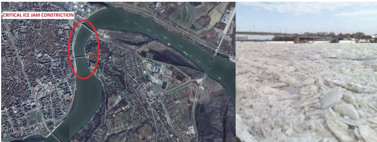
Figure 2 The section of the Danube near Novi Sad (Serbia) experienced an ice jam on February 18, 2012. [6]
