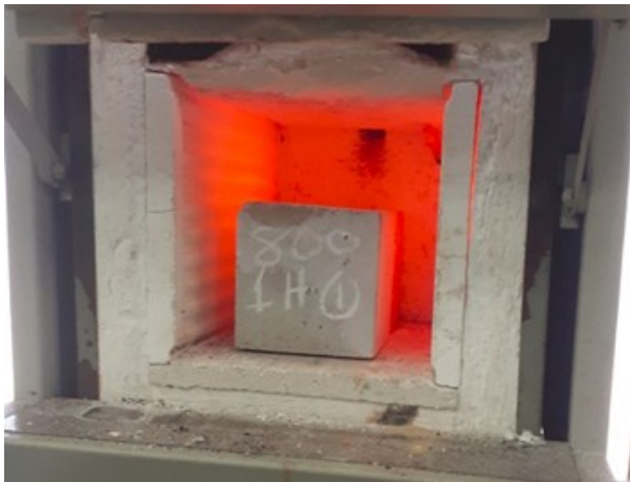
Figure 3. Cube sample in a furnace
