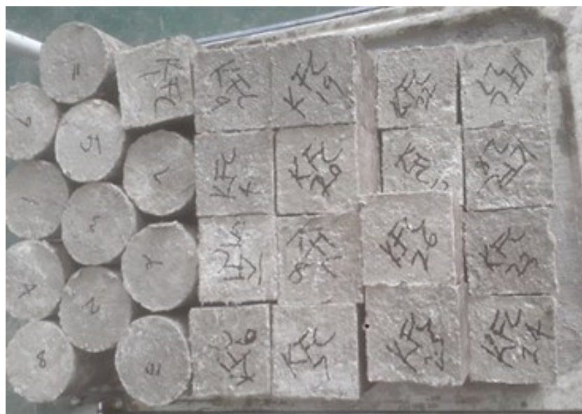
Figure 2. Demoulded cube and cylindrical samples
