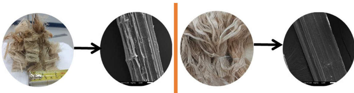
Figure 1. Kenaf fibre: a) treated, b) SEM (treated), c) untreated, and d) SEM (untreated)
