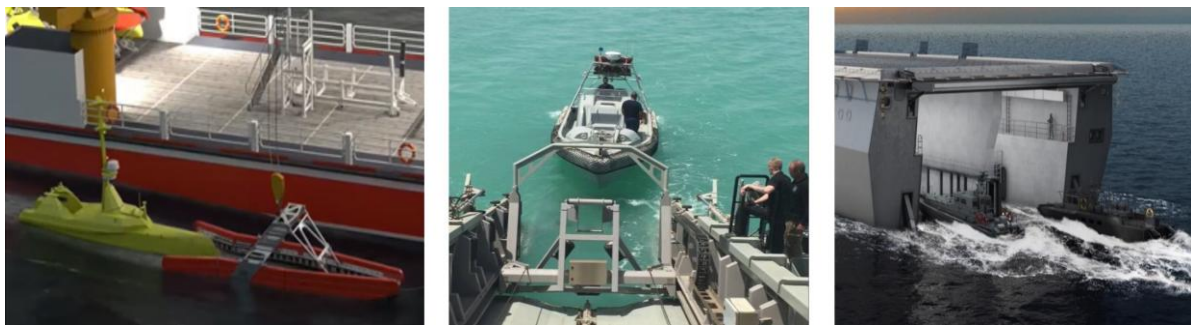
Fig. 1 USV recovery process, left: Lifting type, Middle: Stern Sliding type, right: Docking Bay type
