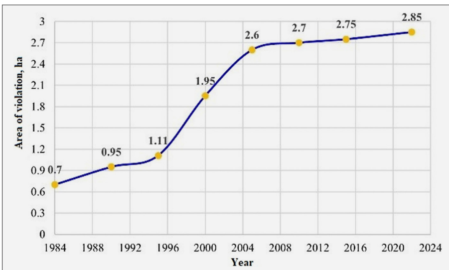
Figure 5. Dynamics of changes in the area of the disturbed earth surface of sinkhole 3
