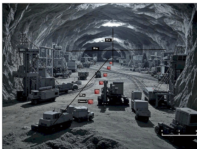
Figure 1. Synthetic underground mine model used for photogrammetric simulation. The 100 m × 50 m × 20 m tunnel network features irregular rock surfaces, mining equipment, and a diffuse lighting gradient (50 lux at center). Red dots indicate camera positions for image capture.
