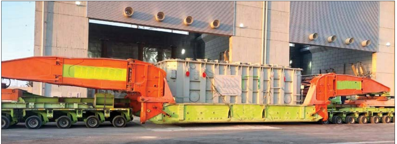
Figure 2a. Transportation of a high-power transformer
